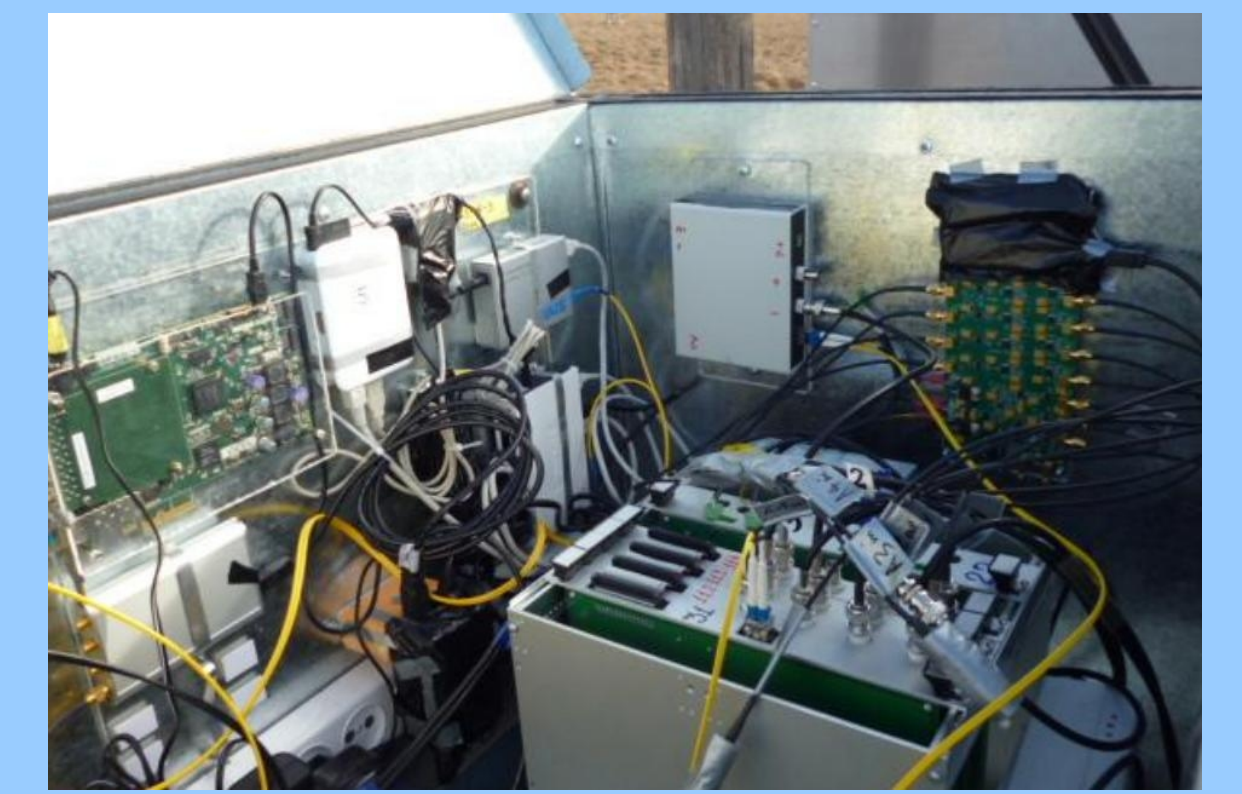
Photo shows a station DAQ: VME crate with Master and FADCs [4], at a distance - summing scheme.
